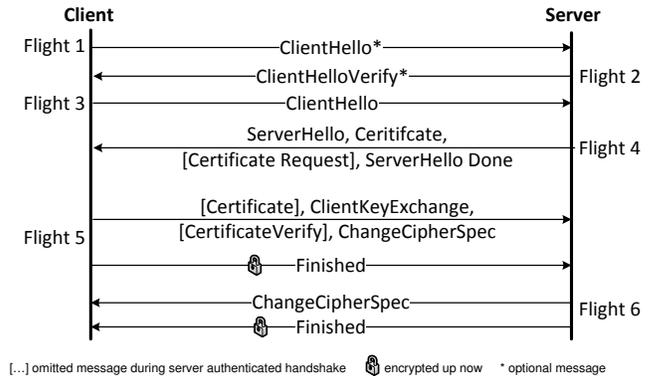
Fig. 2. A fully authenticated DTLS Handshake.
